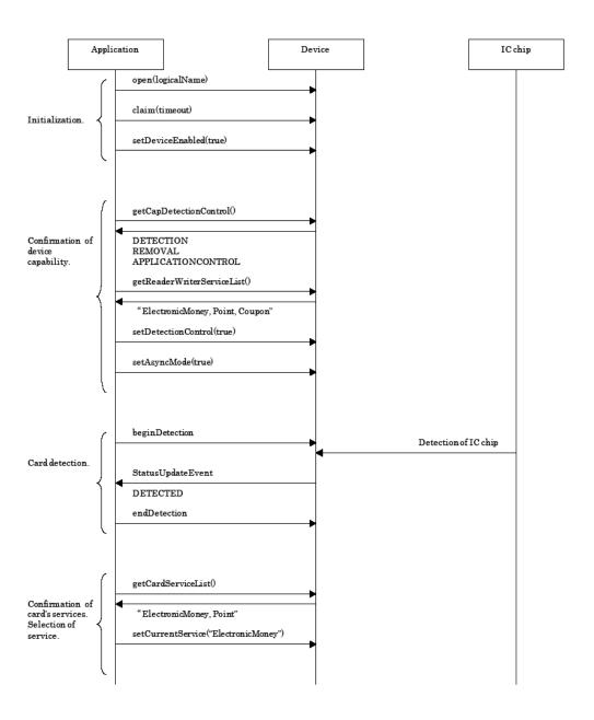
The following sequence diagram shows the continuation of the typical usage of the EVR/W device.
