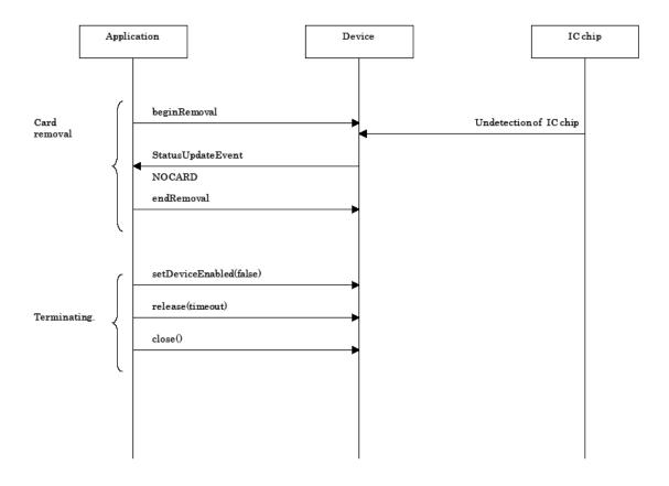
The following sequence diagram shows the CAT(EMV) usage that is used as EVR/W device.
