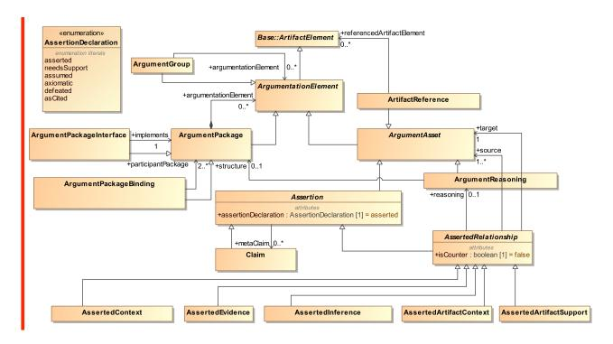
Figure 11.1 - Argumentation Package Diagram
