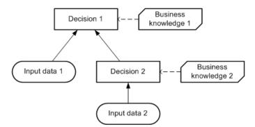
Figure 5.5: A simple Decision Requirements Diagram (DRD)
