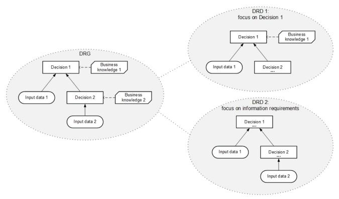
Figure 6.5: DRDs as partial views of a DRG
