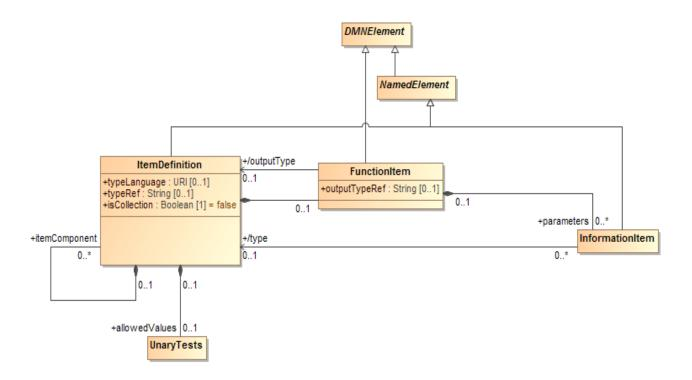
Figure 7.7: ItemDefinition class diagram
