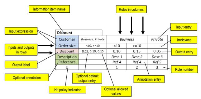
Figure 8.1: Decision table example (vertical orientation: rules as columns)
